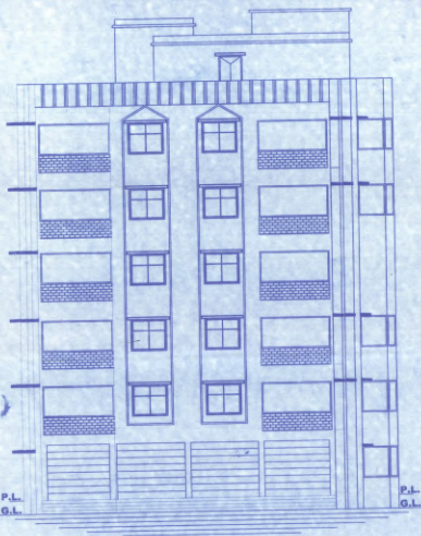
FRONT ELEVATION SCALE = 1:100
