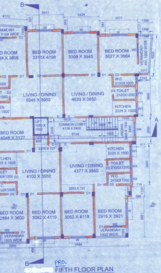
EXISTING FIFTH FLOOR PLAN SCALE = 1:100
